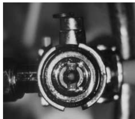
Photo 2. Pitted brass surface of keg coupler
